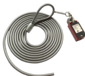
Pull switch with plastic pull cord Horizontal or vertical fitting possible, aluminum die-cast housing IP 65, cord length 4 m
